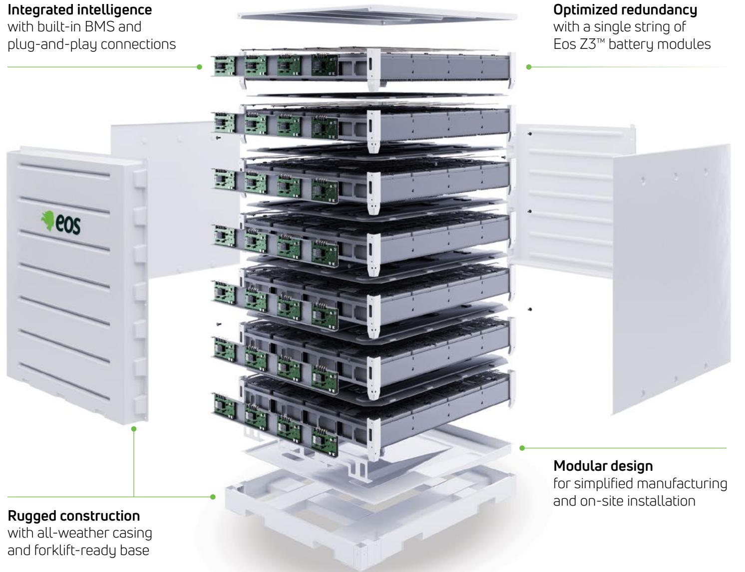
The Indensity Core integrates Eos Z3™ battery modules, the Eos DawnOS™ platform, and onboard cooling fans into a self-contained, modular, and stackable form factor. These compact building blocks enable easier transport, simpler on-site installation, and faster electrical connection—while ensuring a precise fit within the available space, generous spacing for airflow, and clear access for long-term servicing.
